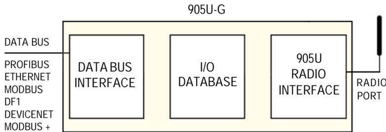
The 905U radio protocol is designed for very efficient radio usage, with configurable communications based on event reporting (I/O change), update times and/or poll response. Other features are:
