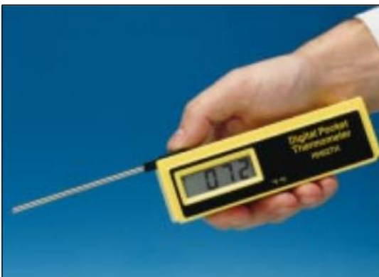
Integral probe allows one-hand operation
